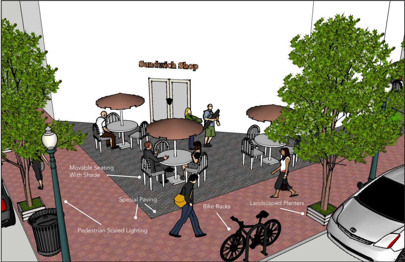
Figure 4.3 Chamfered Corners with outdoor seating
